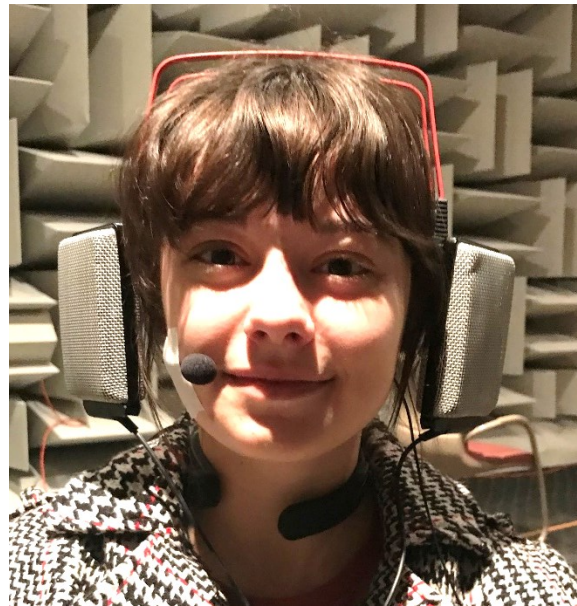
Figure 4.4. A female participant wearing AKG K1000 headphones and a head-worn DPA 4060 microphone. The headphones are offset from the ear, allowing for less disruption of the head diffracted sound. The transducers are angle-adjustable, but may be locked into position
