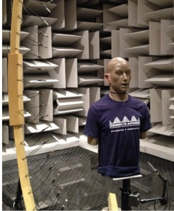
Figure 2.4. KEMAR mannequin centered in arc array for directivity measurements.
