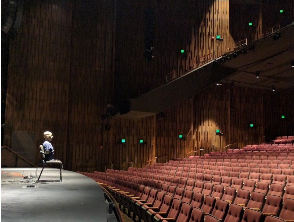
Figure 3.13. KEMAR mannequin positioned near the front of the stage in the de Jong Concert Hall for an OBRIR measurement.
