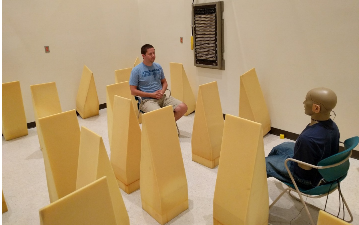
Figure 3.9. KEMAR and researcher positions during an OBRIR measurement in the reverberation chamber. The presence of 32 absorbing wedges in the room reduces the reverberation time and affects the resulting OBRIR.
